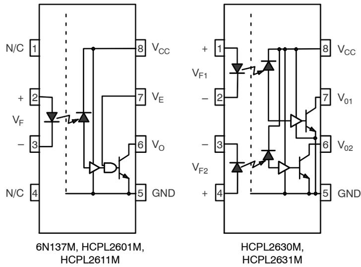
A 0.1  $\mu$ F bypass capacitor must be connected between pins 8 and 5 (Note 1).
