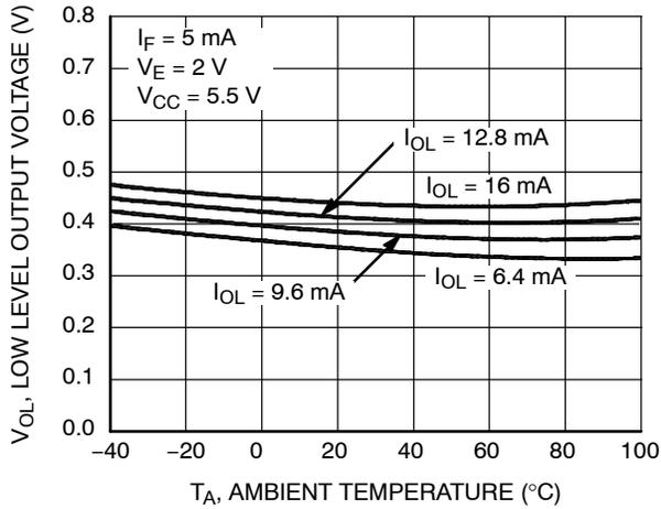
**Figure 2. Low Level Output Voltage vs. Ambient Temperature**
