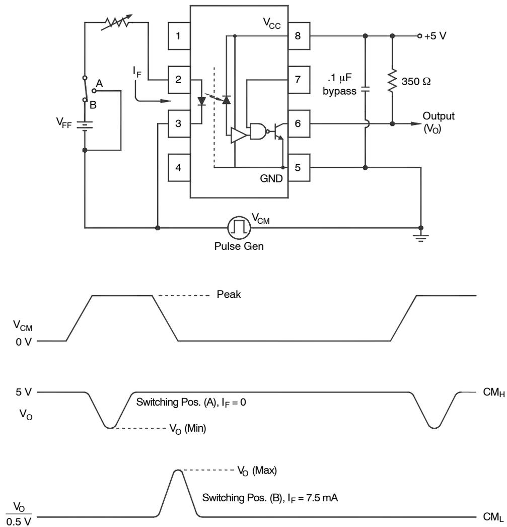
Figure 25. Test Circuit Common Mode Transient Immunity
