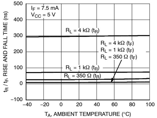
**Figure 9. Rise and Fall Time vs. Temperature**
