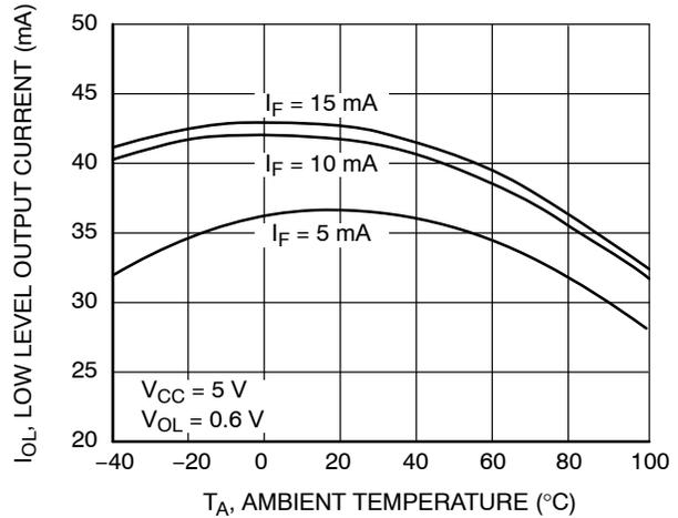
**Figure 16. Low Level Output Current vs. Ambient Temperature**
