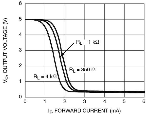
**Figure 18. Output Voltage vs. Input Forward Current**
