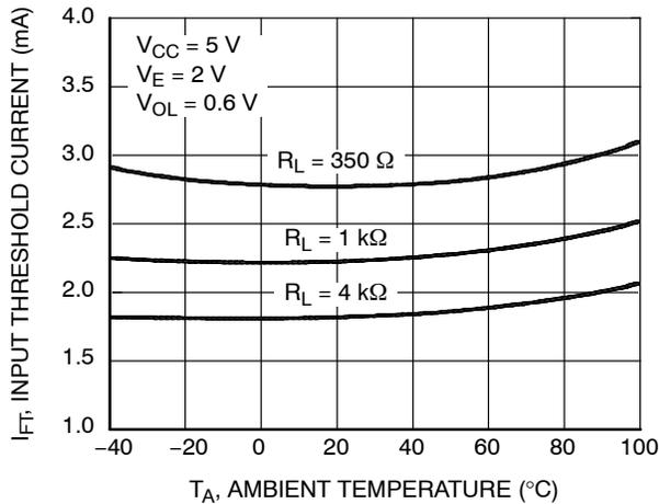
**Figure 6. Input Threshold Current vs. Ambient Temperature**
