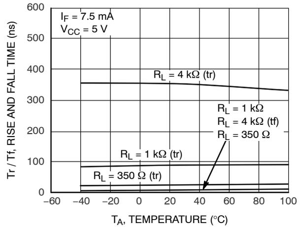
Figure 20. Rise and Fall Time vs. Temperature
