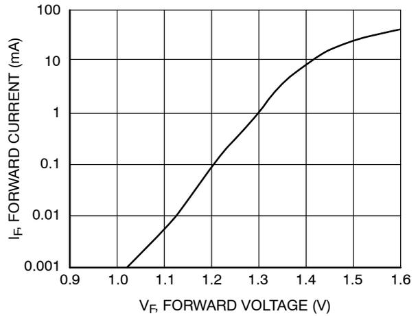
**Figure 14. Input Diode Forward Voltage vs. Forward Current**
