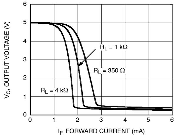
**Figure 7. Output Voltage vs. Input Forward Current**
