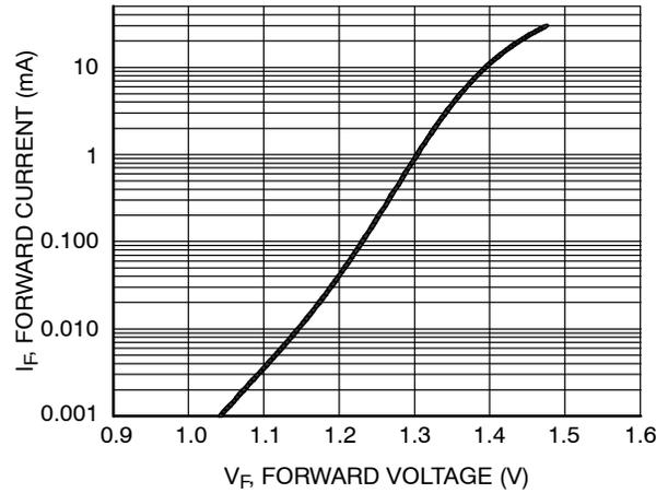
**Figure 3. Input Diode Forward Voltage vs. Forward Current**
