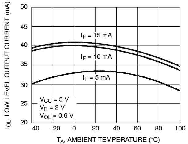
**Figure 5. Low Level Output vs. Ambient Temperature**
