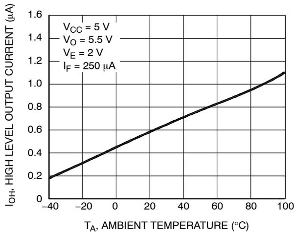
**Figure 12. High Level Output Current vs. Temperature**
