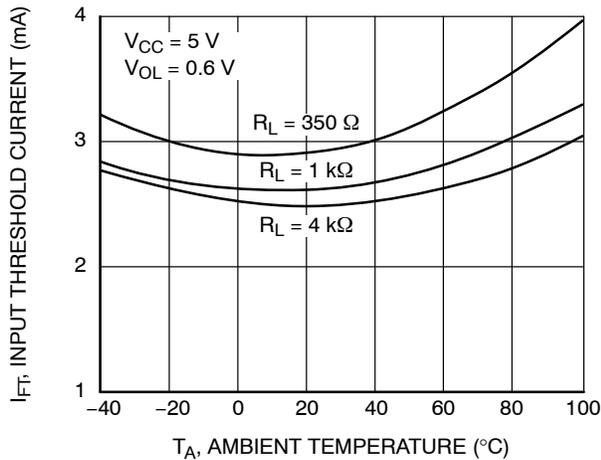
**Figure 17. Input Threshold Current vs. Ambient Temperature**
