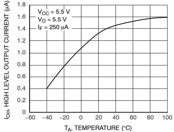
Figure 22. High Level Output Current vs. Temperature
