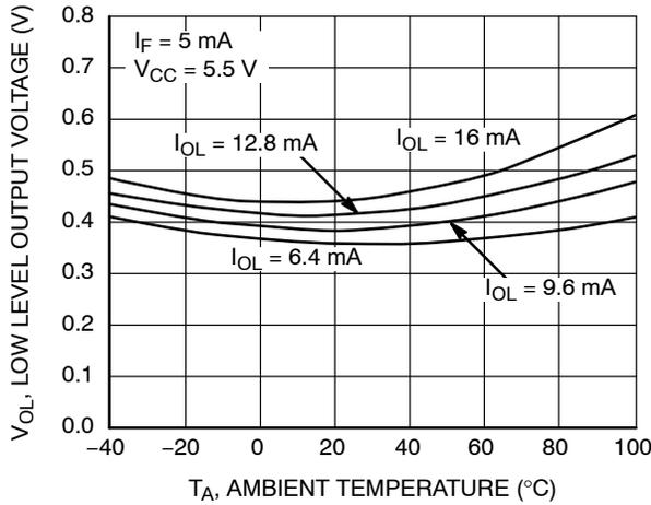
**Figure 13. Low Level Output Voltage vs. Ambient Temperature**
