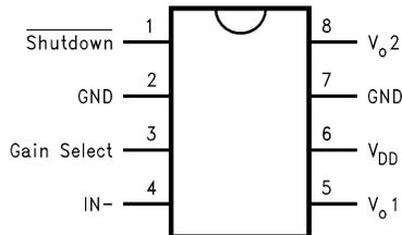
Figure 2. VSSOP Package (Top View)
