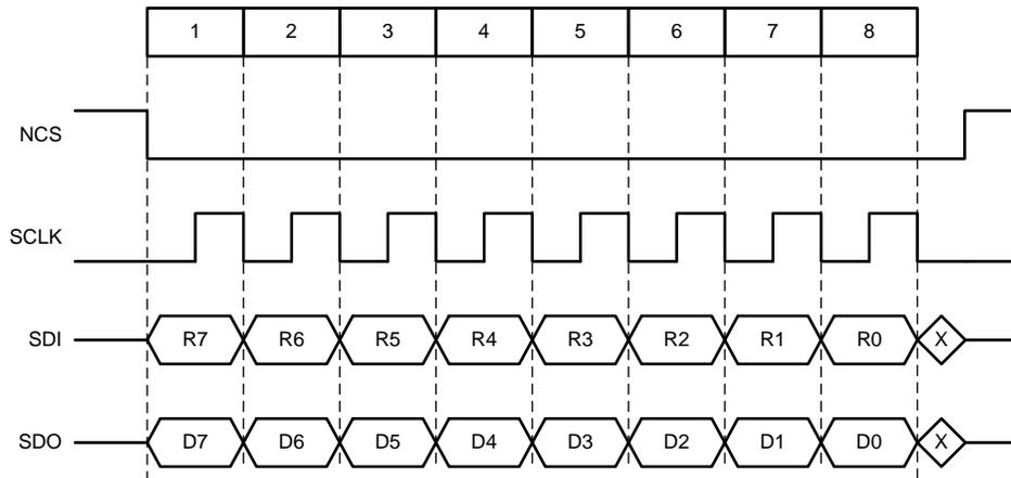
NOTE: SPI master (MCU) and SPI slave (DRV3220-Q1) sample received data on the falling SCLK edge and transmit on the rising SCLK edge.
