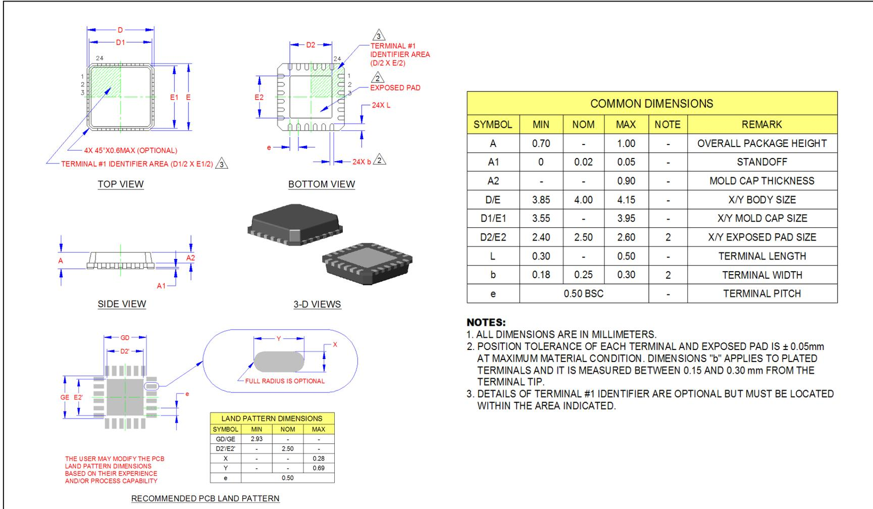
Figure 2 24-Pin QFN, 4x4mm Body, 0.5mm Pitch
