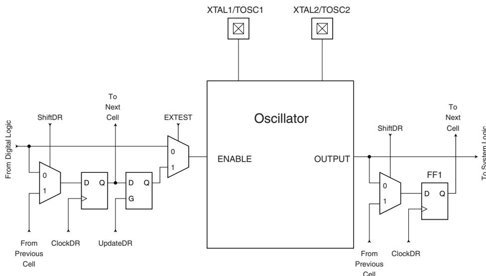
Table 25-3 summarizes the scan registers for the external clock pin XTAL1, Oscillators with XTAL1/XTAL2 connections as well as 32kHz Timer Oscillator.
