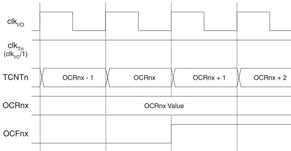
[Figure 17-11](#) shows the same timing data, but with the prescaler enabled.
