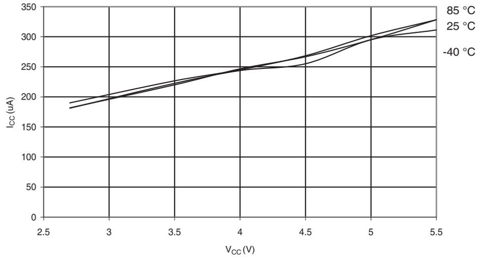
**Figure 29-49. AREF External Reference Current vs.  $V_{CC}$**
