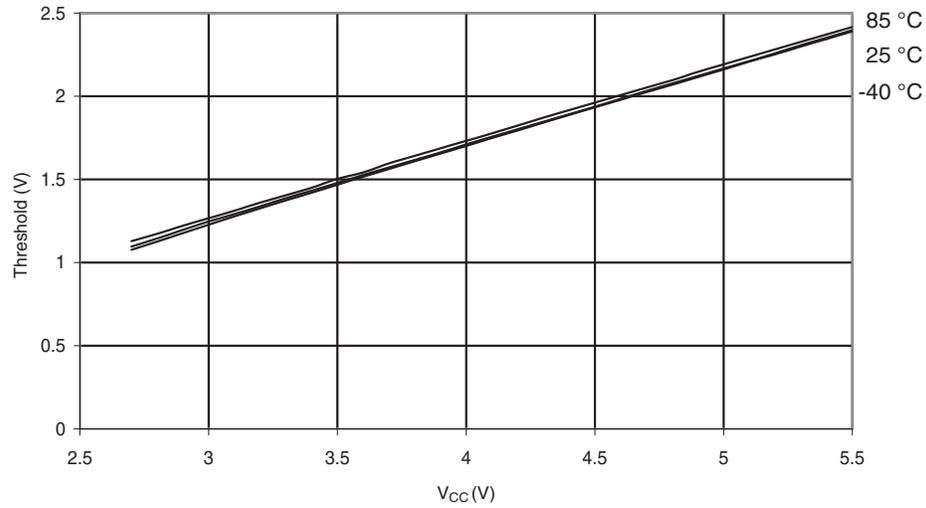
**Figure 29-27. I/O Pin Input Hysteresis vs.  $V_{CC}$**
