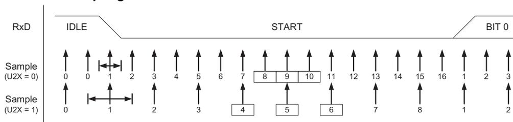
When the clock recovery logic detects a high (idle) to low (start) transition on the RxD line, the start bit detection sequence is initiated. Let sample 1 denote the first zero-sample as shown in the figure. The clock recovery logic then uses samples 8, 9, and 10 for Normal mode, and samples 4, 5, and 6 for Double Speed mode (indicated with sample numbers inside boxes on the figure), to decide if a valid start bit is received. If two or more of these three
