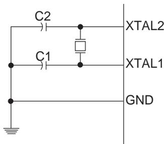
The Oscillator can operate in three different modes, each optimized for a specific frequency range. The operating mode is selected by the fuses CKSEL3:1 as shown in [Table 9-3](#).
