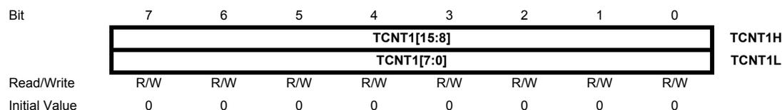
The two *Timer/Counter* I/O locations (TCNT1H and TCNT1L, combined TCNT1) give direct access, both for read and for write operations, to the Timer/Counter unit 16-bit counter. To ensure that both the high and low bytes are read and written simultaneously when the CPU accesses these registers, the access is performed using an 8-bit temporary High Byte Register (TEMP). This temporary register is shared by all the other 16-bit registers. See [“Accessing 16-bit Registers”](#) on page 95.
