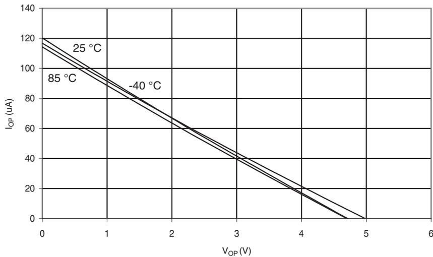
**Figure 29-18. I/O Pin Pull-up Resistor Current vs. Input Voltage ( $V_{CC} = 2.7V$ )**
