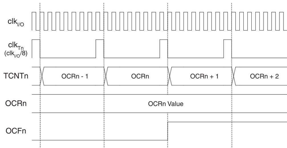
Figure 15-11 shows the setting of OCF0 and the clearing of TCNT0 in CTC mode.
