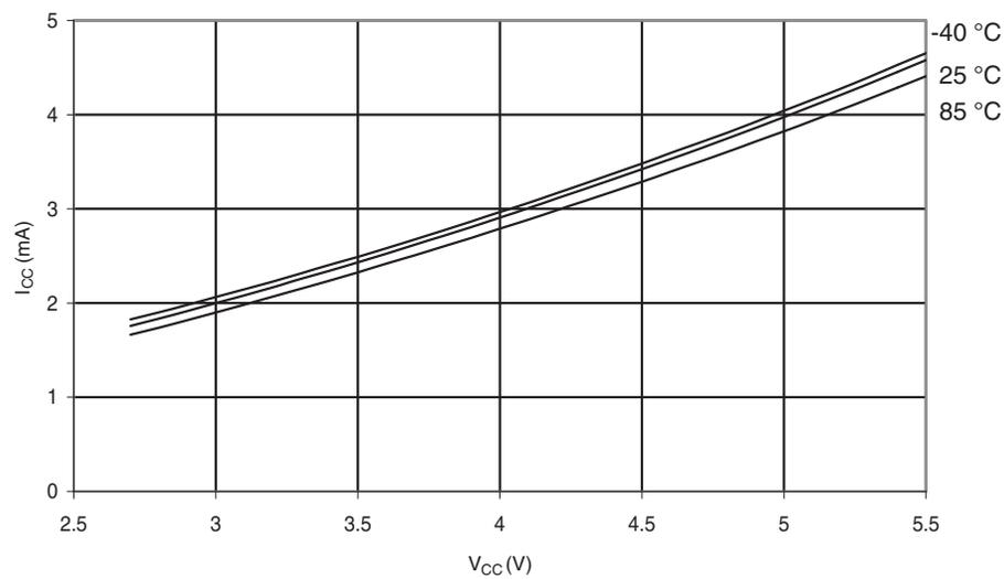
**Figure 29-10. Idle Supply Current vs.  $V_{CC}$  (Internal RC Oscillator, 4MHz)**
