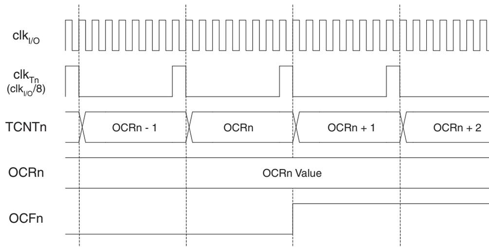
Figure 18-11 shows the setting of OCF2 and the clearing of TCNT2 in CTC mode.
