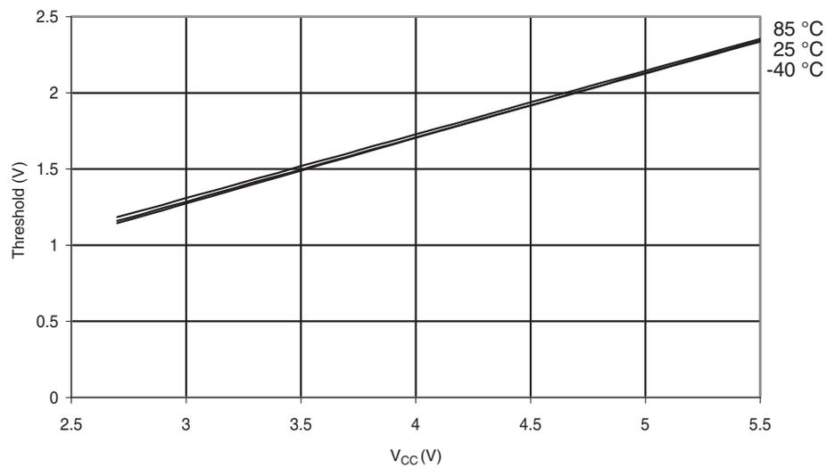
Figure 29-30. Reset Input Pin Hysteresis vs.  $V_{CC}$
