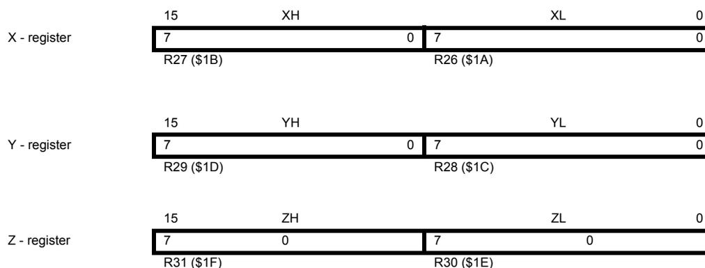
In the different addressing modes these address registers have functions as fixed displacement, automatic increment, and automatic decrement (see the AVR Instruction Set Manual on [www.microchip.com](http://www.microchip.com) for details).
