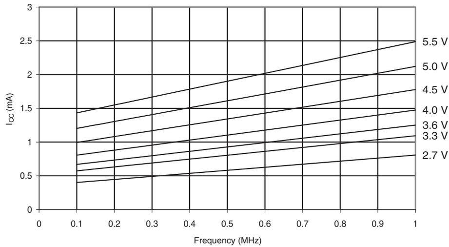
**Figure 29-53. Reset Supply Current vs. Frequency**
