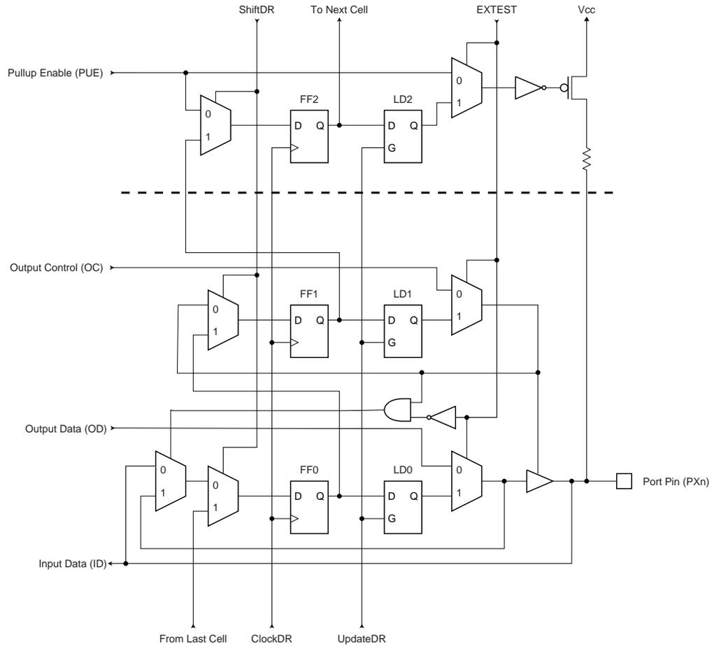
**Figure 25-4. General Port Pin Schematic Diagram<sup>(1)</sup>**
