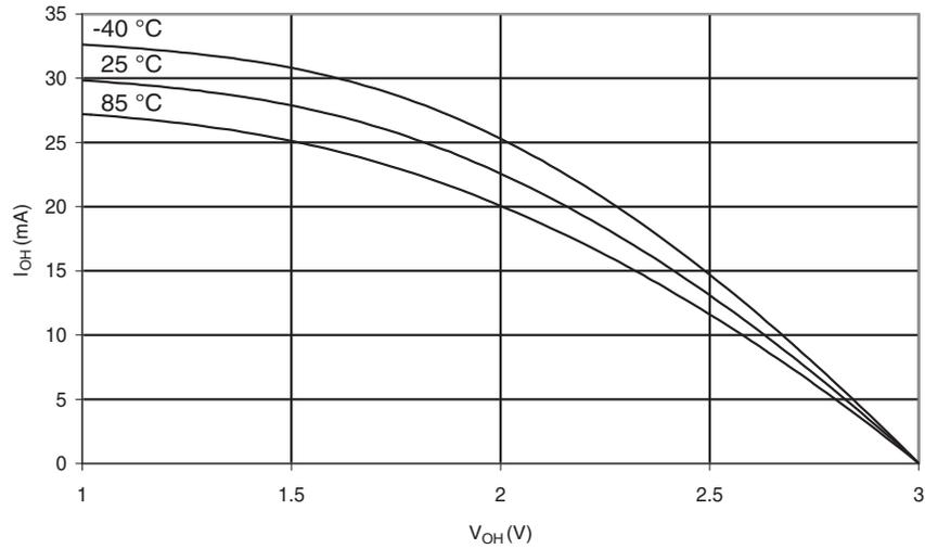
**Figure 29-23. I/O Pin Sink Current vs. Output Voltage ( $V_{CC} = 5V$ )**
