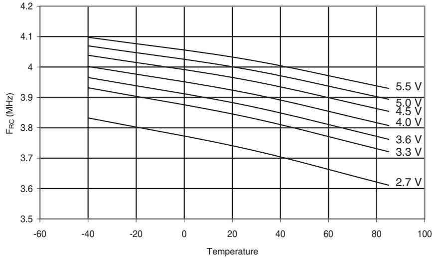
**Figure 29-39. Calibrated 4MHz RC Oscillator Frequency vs.  $V_{CC}$**
