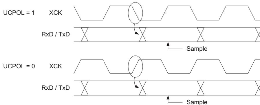
The UCPOL bit UCRSC selects which XCK clock edge is used for data sampling and which is used for data change. As [Figure 20-3](#) shows, when UCPOL is zero the data will be changed at rising XCK edge and sampled at falling XCK edge. If UCPOL is set, the data will be changed at falling XCK edge and sampled at rising XCK edge.
