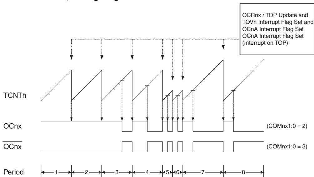
The Timer/Counter Overflow Flag (TOV1) is set each time the counter reaches TOP. In addition the OC1A or ICF1 Flag is set at the same timer clock cycle as TOV1 is set when either OCR1A or ICR1 is used for defining the TOP value. If one of the interrupts are enabled, the interrupt handler routine can be used for updating the TOP and compare values.
