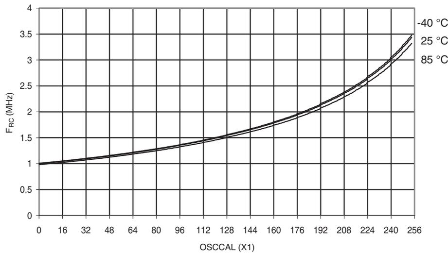
**Figure 29-44. Calibrated 1MHz RC Oscillator Frequency vs. Temperature**
