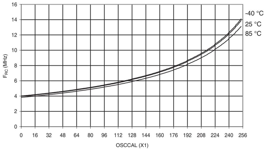
**Figure 29-38. Calibrated 4MHz RC Oscillator Frequency vs. Temperature**
