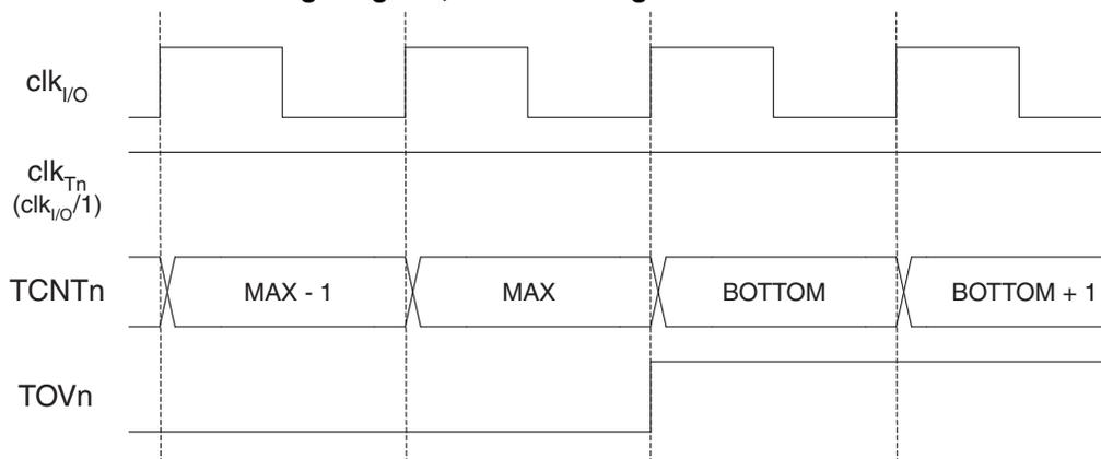
[Figure 18-9](#) shows the same timing data, but with the prescaler enabled.
