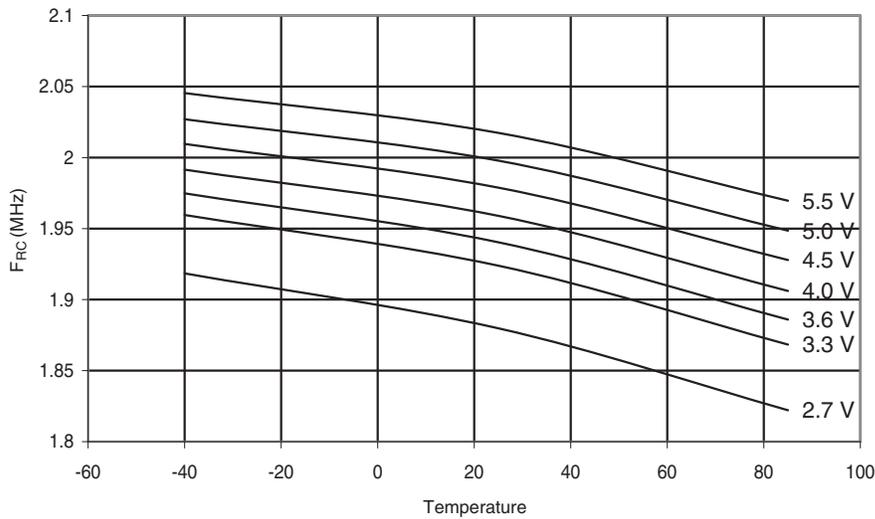
**Figure 29-42. Calibrated 2MHz RC Oscillator Frequency vs.  $V_{CC}$**
