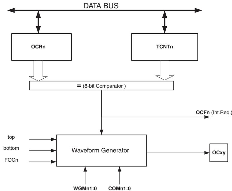
The OCR2 Register is double buffered when using any of the Pulse Width Modulation (PWM) modes. For the normal and Clear Timer on Compare (CTC) modes of operation, the double buffering is disabled. The double buffering synchronizes the update of the OCR2 Compare Register to either top or bottom of the counting sequence. The synchronization prevents the occurrence of odd-length, non-symmetrical PWM pulses, thereby making the output glitch-free.
