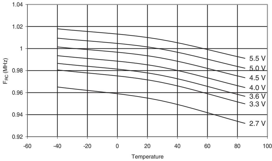
**Figure 29-45. Calibrated 1MHz RC Oscillator Frequency vs. V<sub>CC</sub>**
