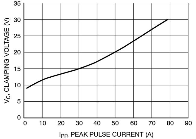
**Figure 4. Clamping Voltage versus Peak Pulse Current**
