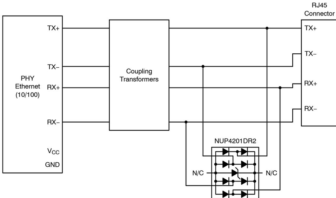
Figure 13. Protection for Ethernet 10/100 (Differential mode)
