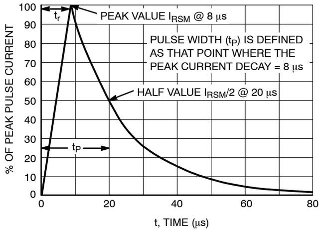
**Figure 3. 8 x 20 µs Pulse Waveform**
