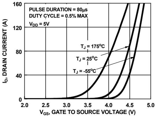
Figure 7. Transfer Characteristics
