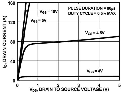
Figure 8. Saturation Characteristics
