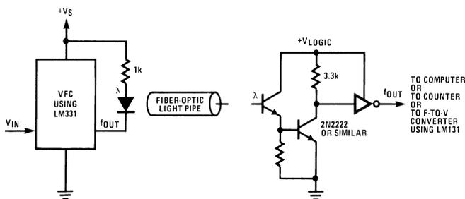
Figure 30. Voltage-to-Frequency Converter With Isolators
