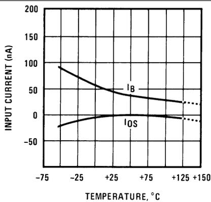
Figure 9. Input Current (Pins 6,7) vs. Temperature
