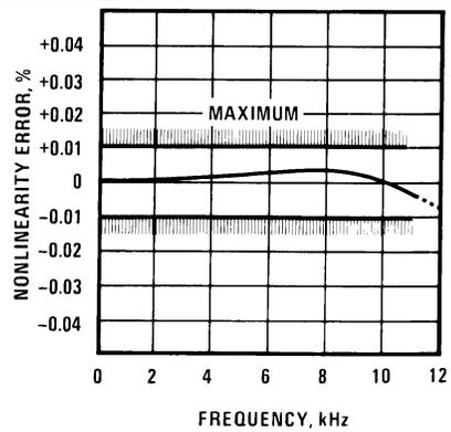
Figure 12. Non-Linearity Error, Precision F-to-V Converter (Figure 19)
