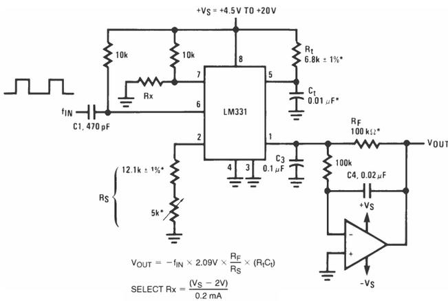
10 kHz Full-Scale With 2-Pole Filter,  $\pm 0.01\%$  Non-Linearity Maximum
