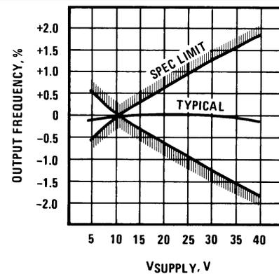
Figure 6. Output Frequency vs.  $V_{SUPPLY}$
