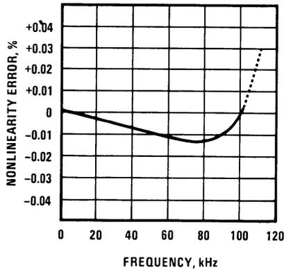
Figure 7. 100 kHz Non-Linearity Error (Figure 17)
