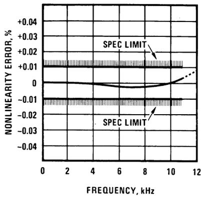
Figure 1. Non-Linearity Error as Precision V-to-F Converter ([Figure 16](#))
