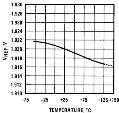
Figure 5.  $V_{REF}$  vs. Temperature
