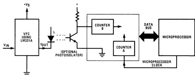
Figure 24. Analog-to-Digital Converter With Microprocessor
