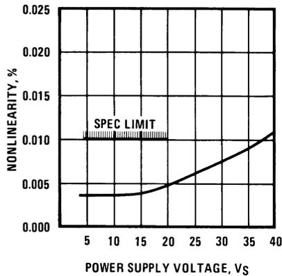
Figure 3. Non-Linearity Error vs. Power Supply Voltage
