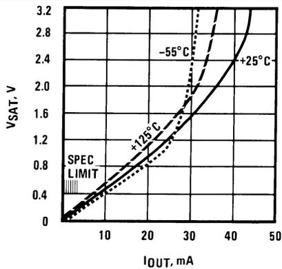
Figure 11. Output Saturation Voltage vs. IOU (Pin 3)
