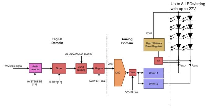
Figure 40. Brightness Control with BRT\_MODE bit 01
