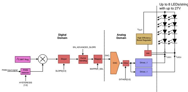
Figure 41. Brightness Control with BRT\_MODE bit 10
