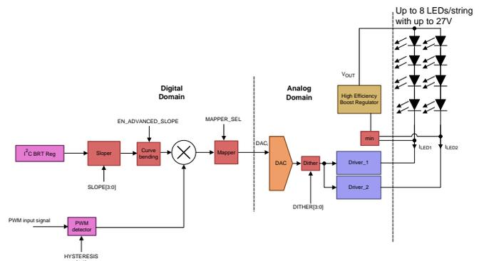
Figure 42. Brightness Control with BRT\_MODE bit 11
