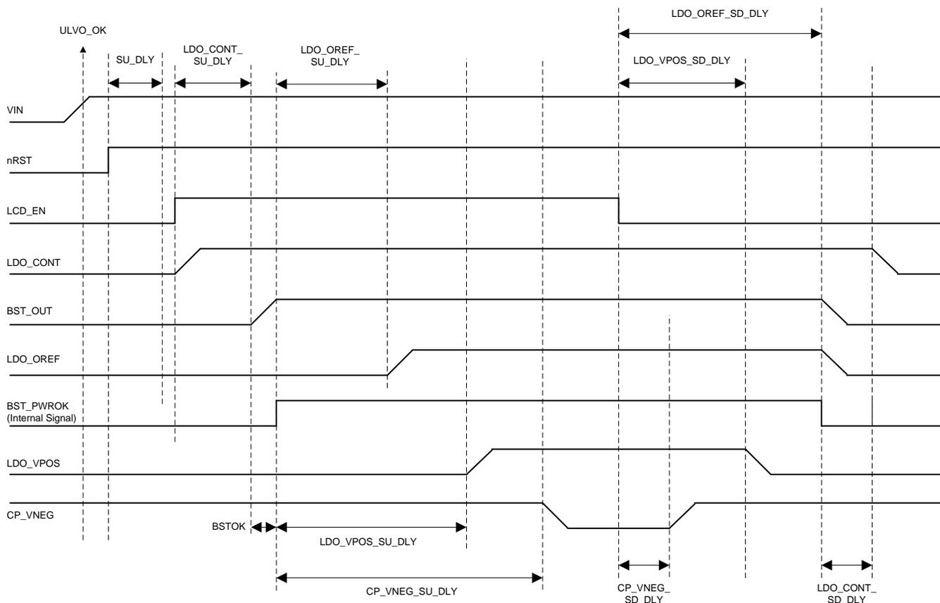
Figure 49. General LCD Bias Power Sequence Without Backlight
