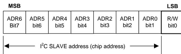
Figure 55. I<sup>2</sup>C Device Address
