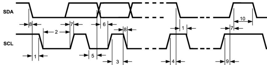
**Figure 1. I<sup>2</sup>C Timing Parameters**
