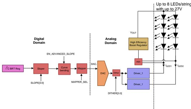
Figure 39. Brightness Control with BRT\_MODE bit 00
