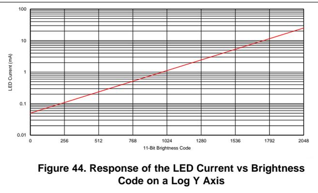
With linear mapping the 11-bit code to current response is approximated by the equation:
