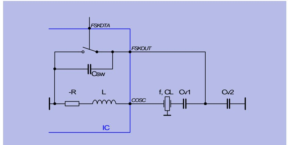
The frequency deviation of the crystal oscillator is multiplied with the divider factor N of the Phase Locked Loop to the output of the power amplifier. In case of small frequency deviations (up to +/- 1000 ppm), the two desired load capacitances can be calculated with the formula below.
