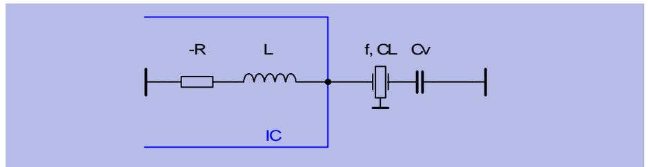
$$C_v = \frac{1}{\frac{1}{C_L} + \omega^2 L} \quad (1)$$
