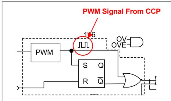
There are two modes of operation that concern the system clock PWM signal. These modes are Stand-Alone (nonfrequency synchronization) and Frequency Synchronization.
