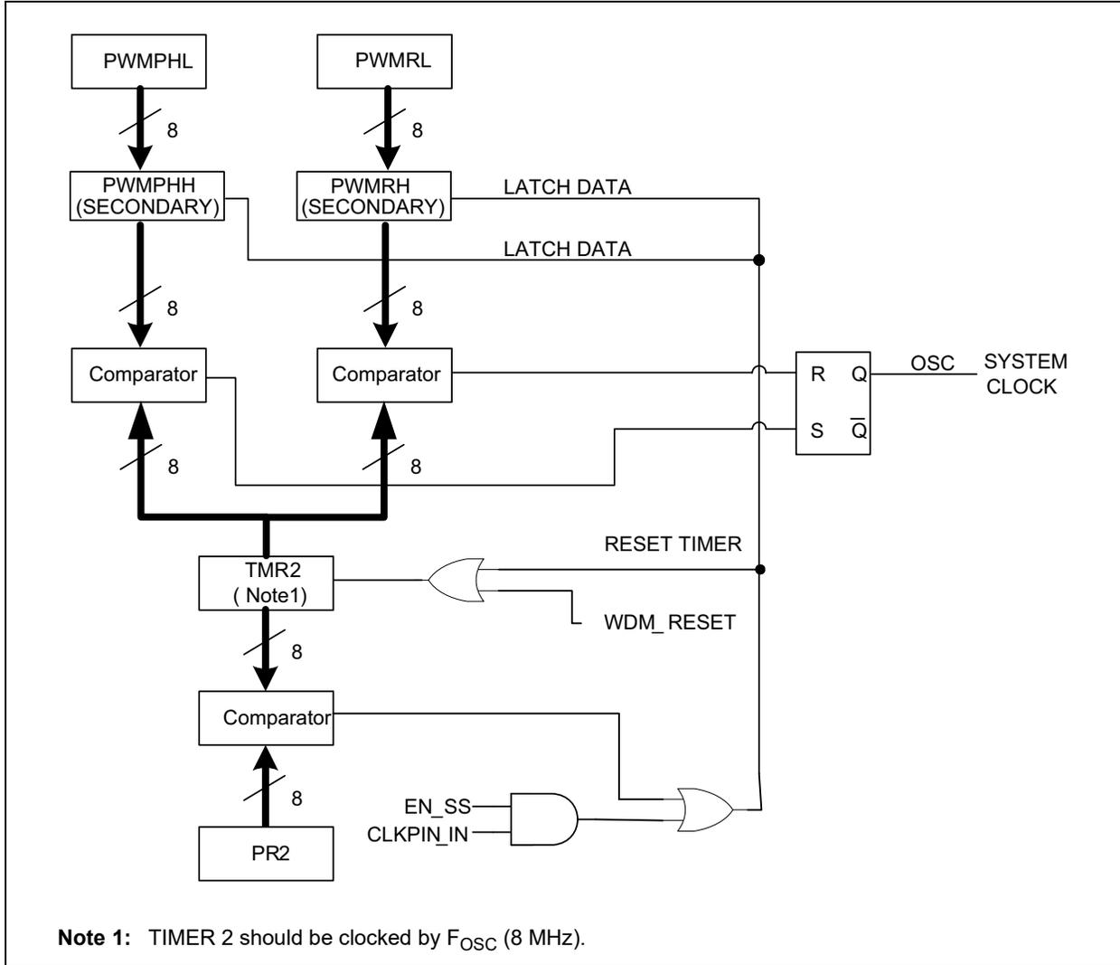
A PWM output (Figure 25-3) has a time base (period) and a time that the output stays high (duty cycle). The frequency of the PWM is the inverse of the period (1/period).
