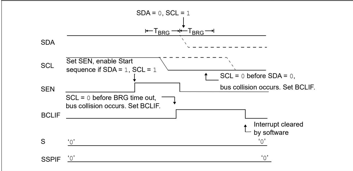
**FIGURE 28-27: BRG RESET DUE TO SDA ARBITRATION DURING START CONDITION**
