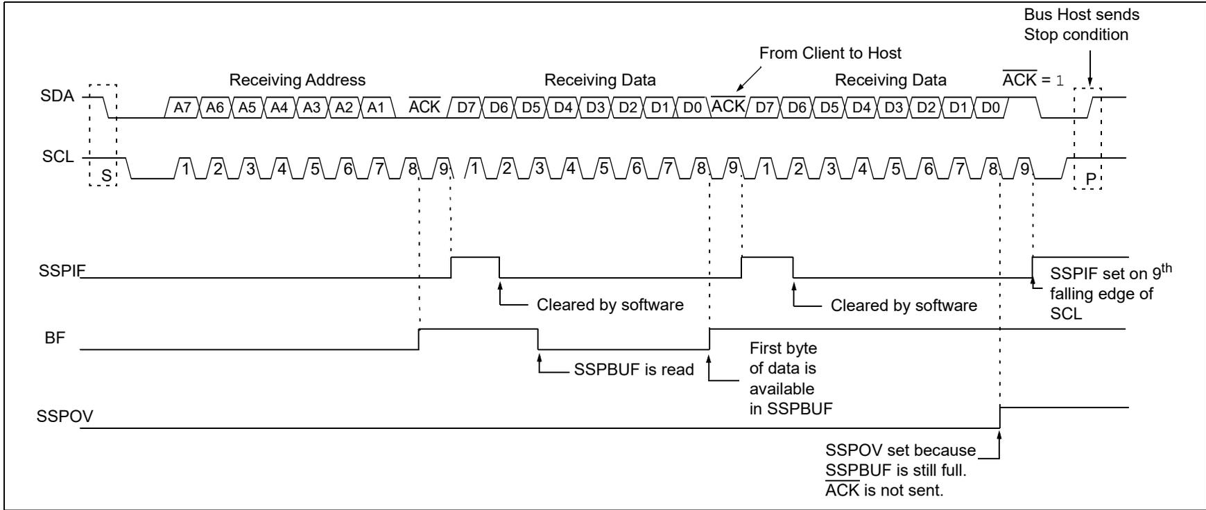
**FIGURE 28-7: I<sup>2</sup>C CLIENT, 7-BIT ADDRESS, RECEPTION (SEN = 1, AHEN = 0, DHEN = 0)**
