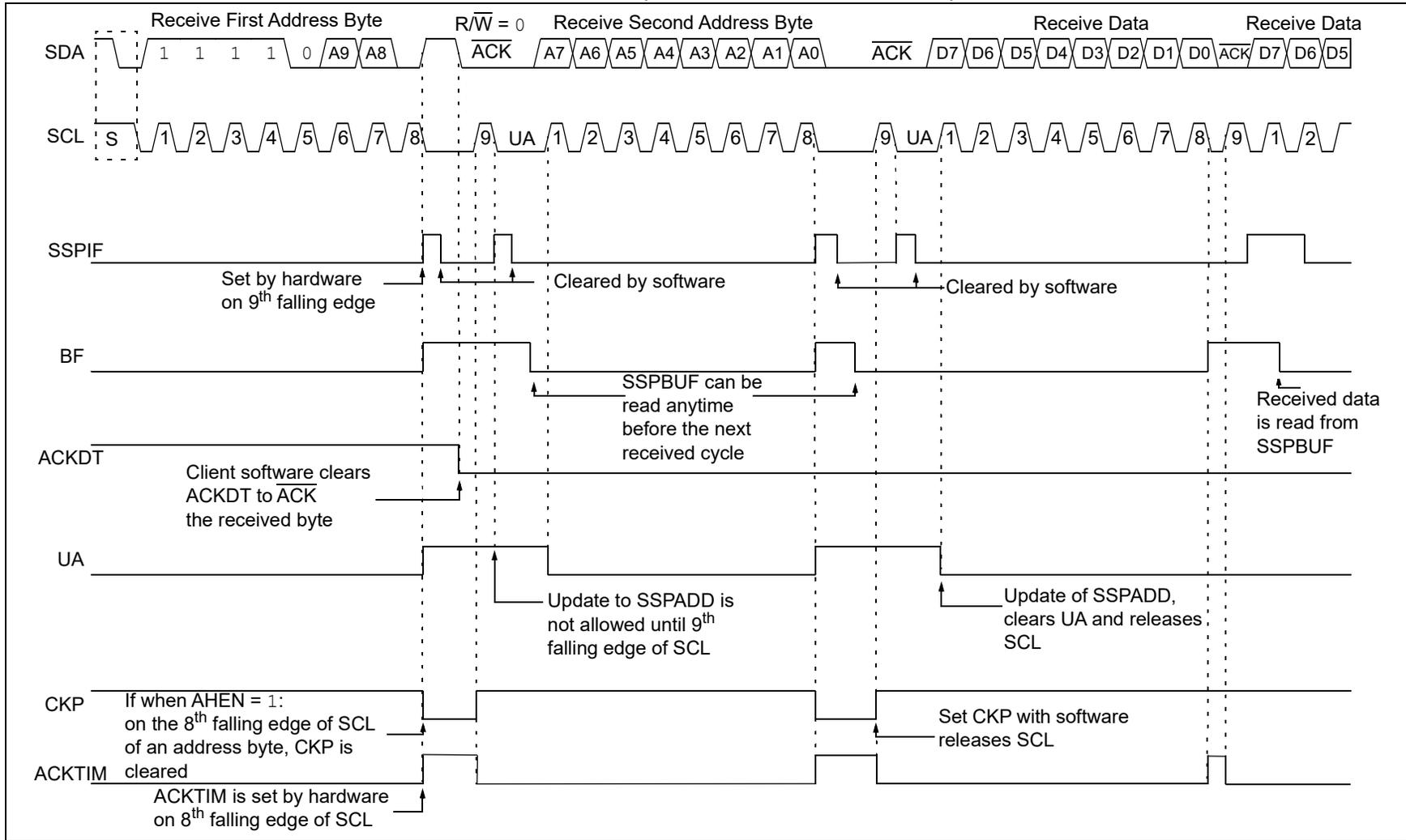
**FIGURE 28-14: I<sup>2</sup>C CLIENT, 10-BIT ADDRESS, TRANSMISSION (SEN = 0, AHEN = 0, DHEN = 0)**
