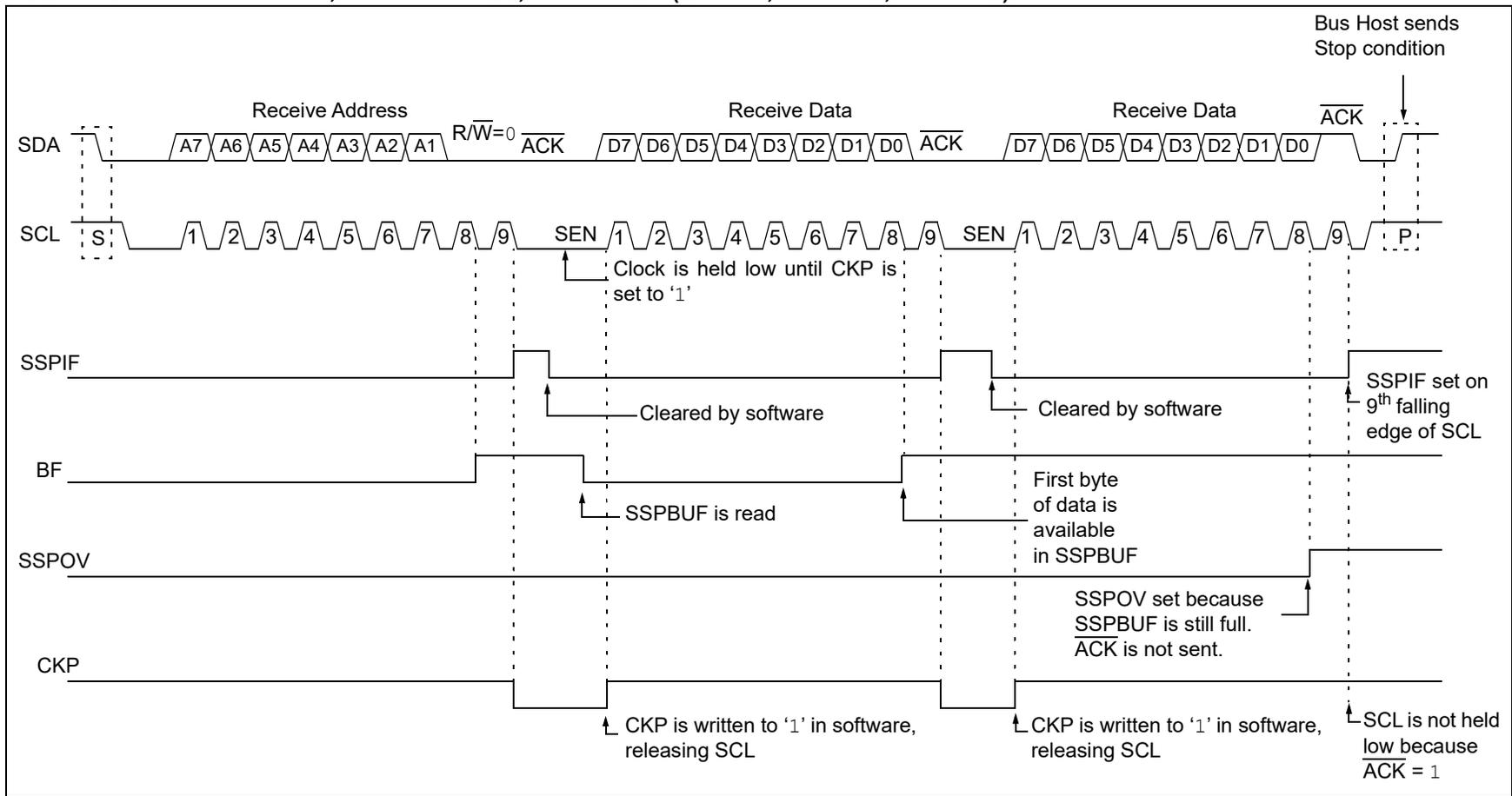
**FIGURE 28-8: I<sup>2</sup>C CLIENT, 7-BIT ADDRESS, RECEPTION (SEN = 0, AHEN = 1, DHEN = 1)**
