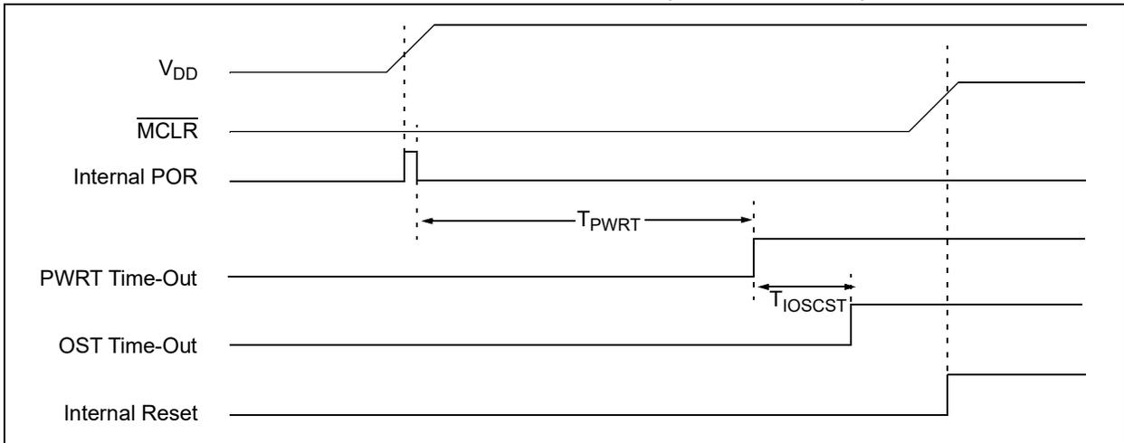
**FIGURE 13-6: TIME-OUT SEQUENCE ON POWER-UP (MCLR WITH V<sub>DD</sub>)**
