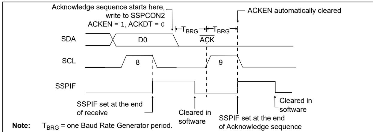
**FIGURE 28-23: STOP CONDITION RECEIVE OR TRANSMIT MODE**
