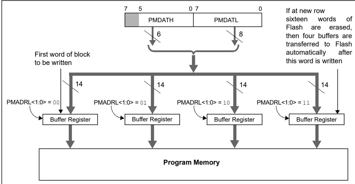
**FIGURE 17-3: FLASH PROGRAM MEMORY LONG WRITE CYCLE EXECUTION**
