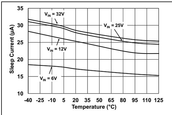
**FIGURE 7-2:**  $I_Q$  vs. Temperature in Sleep Mode.
