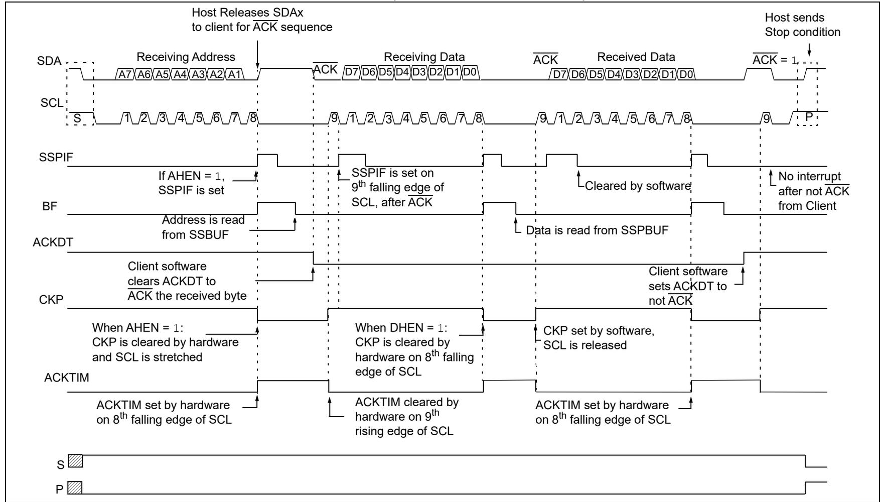
**FIGURE 28-9: I<sup>2</sup>C CLIENT, 7-BIT ADDRESS, RECEPTION (SEN = 1, AHEN = 1, DHEN = 1)**
