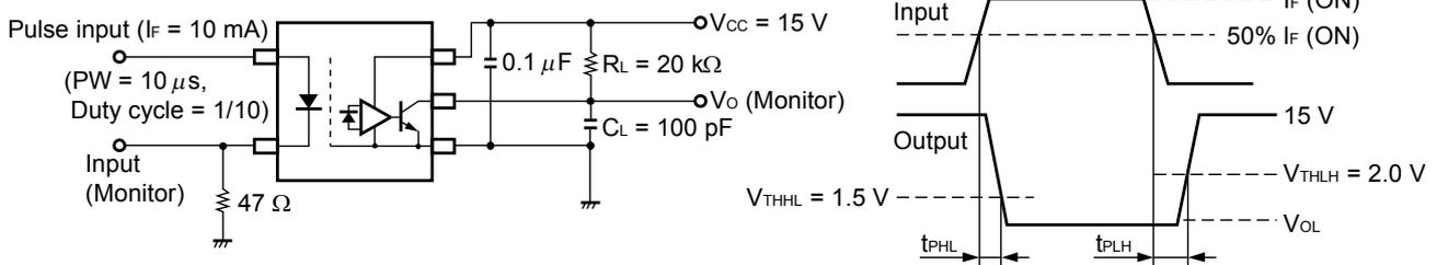
$C_L$  includes probe and stray wiring capacitance.
