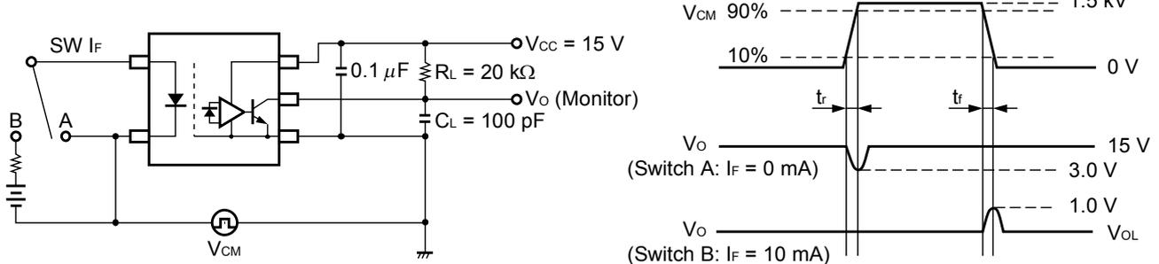
$C_L$  includes probe and stray wiring capacitance.
